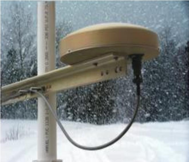
**HIP -100 Hail and Ice Pellet Sensor** is an acoustic sensor developed as an add-on option to OSi's OWI-430 series Weather Sensor, giving an even greater range of weather data collection.
